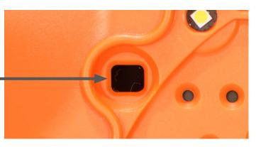
The integrated thermal imaging camera is located next to the microphone array.
